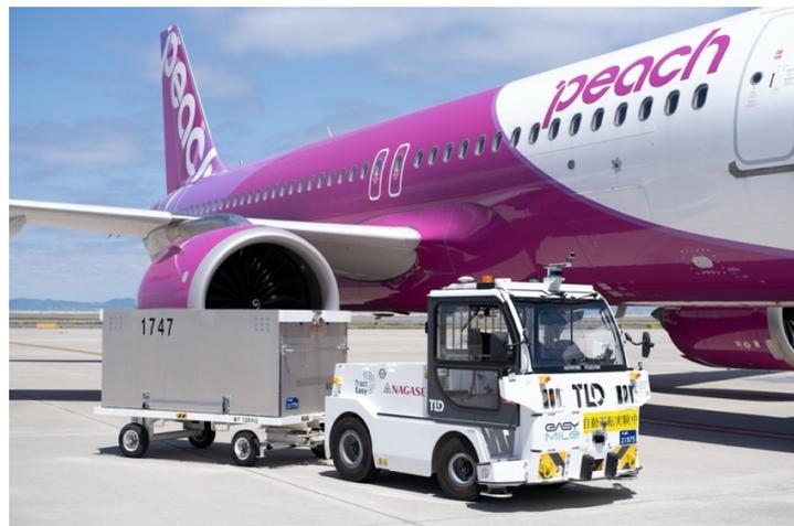
This demonstration test aims to verify the practicality of vehicle operation using autonomous driving technology within the ramp area—marking the first such initiative at Kansai Airport. The trial uses the “EZTow” vehicle manufactured by Tracteas, provided by Nagase Techno. Level 3 autonomous driving test has been conducted from December 2024 through April 20, 2025, and a Level 4 autonomous driving test is currently underway\*<sup>2</sup>.
