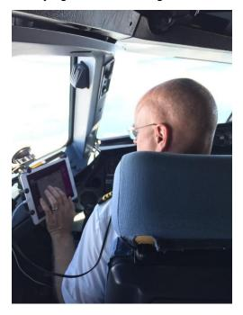
Peach will leverage EFBs that use tablet computer to digitalize printed manuals and other text used in the cockpit, which will enable (its flight crew) to share information on changes in manuals promptly on their tablets, as well as conduct computer calculations on aircraft performance during takeoff and landing to optimize operational efficiency.
