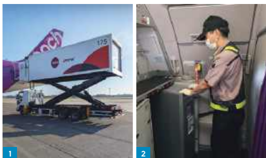
1. Freshly prepared meals are loaded onto the back of a truck and transported overland to the airport. When it's time to board, the truck is raised to the level of the aircraft and connected to the entrance. 2. The carts carrying the fresh meals are brought onto the aircraft and placed in the coolest area. Everything is packed compactly into each cart, like a puzzle.
