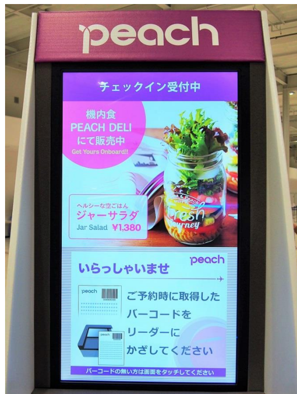
"The size of the monitor screen has been increased from 15 inches to 32 inches, enabling the top and bottom parts to be split as desired and to show different details."
